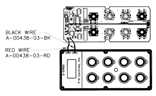
PREPARE AND SOLDER THE BATTERY WIRES FROM THE BATTERY TERMINALS TO THE PC BOARD AS SHOWN.
