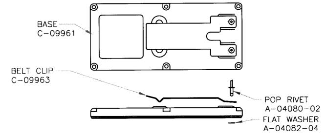
POT RIVET THE BELT CLIP TO THE BASE USING THE PARTS SHOWN.
