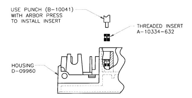
INSTALL AN INSERT, WITH AN ARBOR PRESS, FLUSH OR SLIGHTLY BELOW INTO THE HOUSING AS SHOWN.
