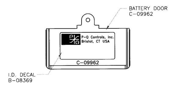
CLEAN DECAL APPLICATION AREA WITH DENATURED ALCOHOL. REMOVE THE ADHESIVE BACKING FROM THE DECAL, AND APPLY THE DECAL TO THE BATTERY DOOR AS SHOWN.
