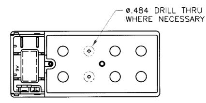
ON HOUSINGS NEEDING MORE SWITCH POSITIONS, DRILL OUT THE HOLES NEEDED BY CENTERING THE DRILL OVER THE COUNTER BORE AND DRILLING OUT THE HOLES IN THE POSITIONS NEEDED.
