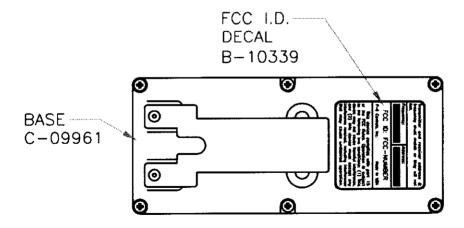
REMOVE THE ADHESIVE BACKING FROM THE DECAL, AND APPLY THE DECAL TO THE BASE AS SHOWN.
