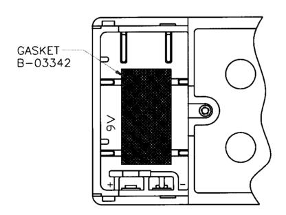
CLEAN GASKET AREA WITH DENATURED ALCOHOL. REMOVE ADHESIVE BACKING FROM THE GASKET, AND APPLY THE GASKET TO THE HOUSING AS SHOWN.
