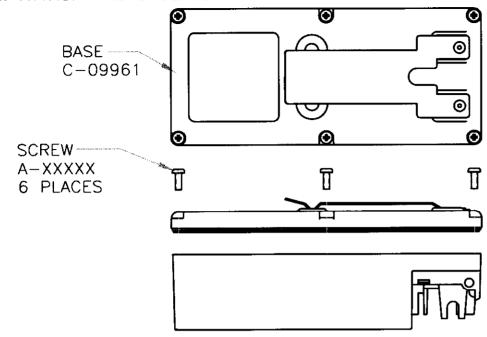
ATTACH THE BASE ASSEMBLY TO THE HOUSING ASSEMBLY WITH THE SCREWS AS SHOWN. TIGHTEN SCREW TO A NOMINAL TORQUE OF: XX in-Ib AND AN ACCEPTABLE RANGE OF: XX in-Ib MIN. AND: XX in-Ib MAX.
