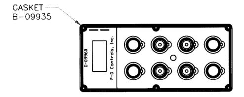
CLEAN GASKET CAVITY WITH DENATURED ALCOHOL REMOVE ADHESIVE BACKING FROM THE GASKET, AND APPLY THE GASKET TO THE HOUSING AS SHOWN.
