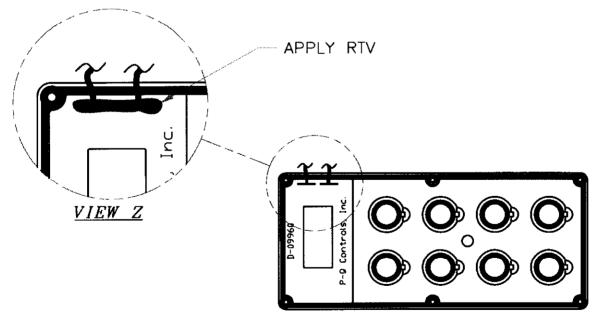
APPLY LOCTITE SELF LEVELING RTV #5140 TO THE CONTACTS AS SHOWN IN VIEW Z. THE OBJECTIVE OF THE RTV IS TO SEAL THE SPACE BETWEEN THE CONTACTS AND THE SLOTS IN THE HOUSING.
