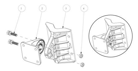
STEP 1: Assemble the Mounting Bracket Set
