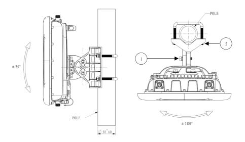
There is a  $\pm$ 30 degrees up/down tilt angle for the mounting bracket.
