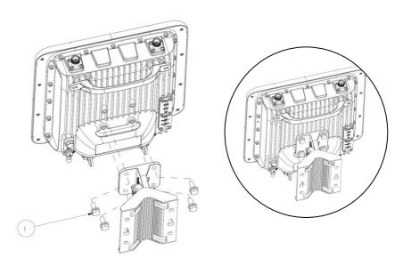
Attach the mounting bracket to the X30 with four M8 hexagon bolts (item 1) with a torque value of 12-15 Nm.
