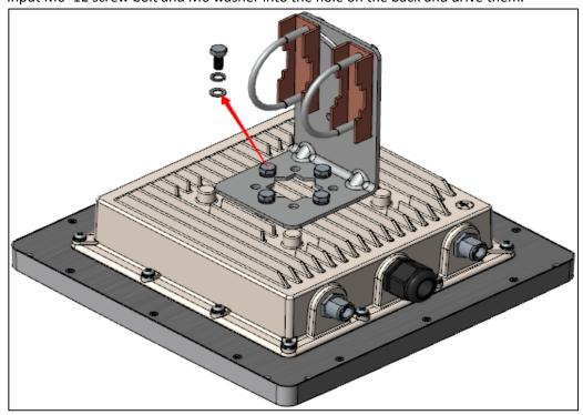
5. Finally mount the AP on the pole as shown in the picture. And drive the screw nut tight with wrench.
