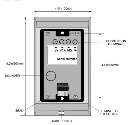
The reader is designed to be surface mounted onto a flat surface using the two holes provided, therefore not requiring the installation of a back box. The readers performance is unaffected by the material of the mounting surface. Ensure the surface is as even as possible to provide maximum protection against the reader being levered from the wall.
