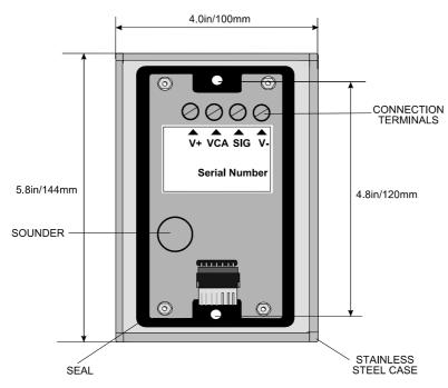
This reader is designed to be flush mounted onto a standard 2 gang (1.4in/35mm) back box using the two M3.5 (1in/25mm x 0.14in/3.5mm) screws provided.
