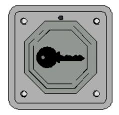
The KeyPAC Vandal (PAC Part Number 20450 or K3002) proximity reader is an accessory commonly used on a majority of access control systems. The Vandal uses pre-encoded ISO proximity cards (PAC Part Number 21030). Each card is encoded with a unique code that outputs a serial number to the access control system.
