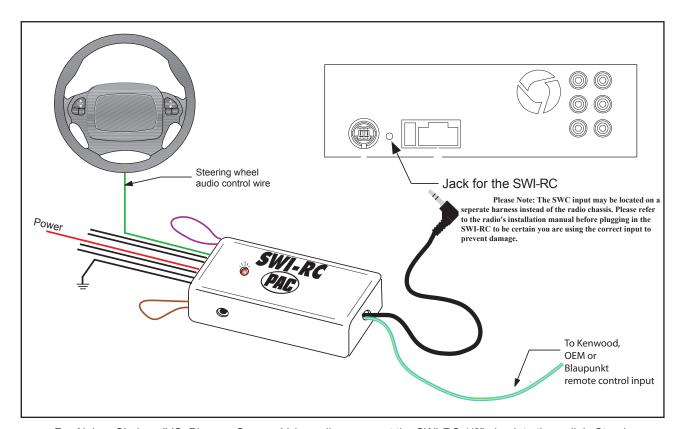
For Alpine, Clarion, JVC, Pioneer, Sony or Valor radios, connect the SWI-RC 1/8" plug into the radio's Steering Wheel input jack on back of radio or wire harness. For Kenwood or OEM radios, connect the blue/yel wire to the remote Input wire (blue/yel or yel/blu for Kenwood, gray for OEM) of radio.
