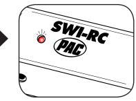
Once programming is completed, **wait 7 seconds**. The LED will flash three times indicating end of programming. The Interface will then flash the vehicle version number it was programmed for.
