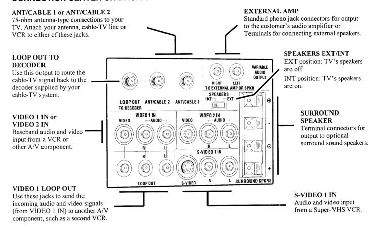
Some connections require additional cables or equipment which are not supplied with the TV.
