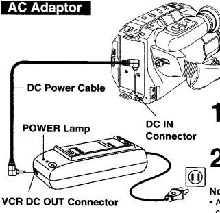
Connect AC Adaptor VCR DC OUT to Camcorder DC IN with supplied DC Power Cable.
