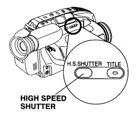
Press HIGH SPEED SHUTTER while recording.
