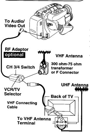
If TV has no VIDEO/AUDIO IN jacks, connect <u>PV-RF16 RF Adaptor</u> (optional). Tune TV to CH 3 or 4 to match RF Adaptor 3/4 switch. Set Adaptor's TV/VCR switch to VCR for playback.
