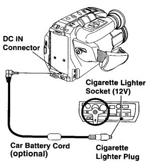
Connect PV-C16 <u>Car Battery Cord</u> (optional) to <u>Camcorder DC IN</u>.
