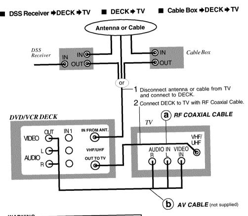
When using "Nut type" RF coaxial cables, tighten with fingers only. Overtightening may damage terminals.
