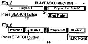
Fig.3 If search exceeds a few seconds in BLANK area. Press SEARCH button
