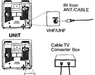
WARNING: Overtightening "Nut type" RF coaxial cables may damage jacks. Finger tighten only.
