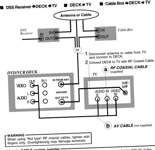
Note to CABLE system installer This reminder is provided to call the CABLE system installer's attention to Article 820-40 of the NEC in USA (and to the Canadian Electrical Code in Canada) that provides guidelines for proper grounding and, in particular, specifies that the cable ground shall be connected to the grounding system of the building, as close to the point of cable entry as practical.
