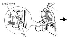
Open the lock cover while pinching the protection portion of both ends.
