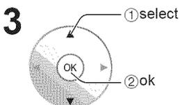
Press **▲▼** to highlight a position on the list. Then, press **OK** to save the displayed channel in that position.
