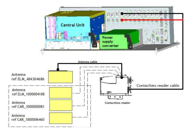
Only 4 different antennas can be integrated (ref ELM\_404304686/ ELM\_1000004108 / CAR\_1000000081 / CAR\_1000006460)
