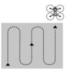
according to the itinerary displayed on the screen. **Polygon**:the drone performs a grid flight of the area
