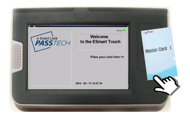
Place Master Card on the controller to set the functions to operate the locks through controller.
