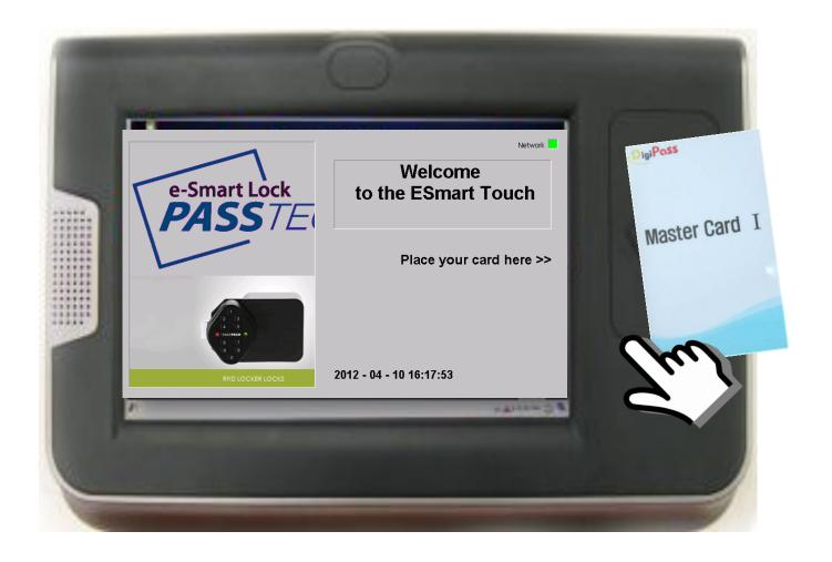
Place MASTER CARD on the controller twice to register user cards & assign locks as well as opening locks with a master card at an emergency.
