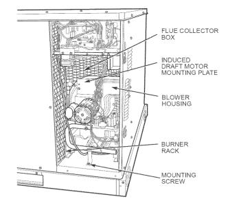
Fig. 24 — Blower Housing and Flue Collector Box
