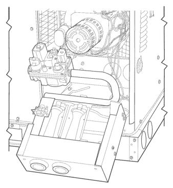
Fig. 27 — Burner Rack Removed
