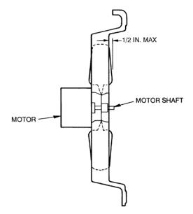
Fig. 18 — Fan Blade Clearance
