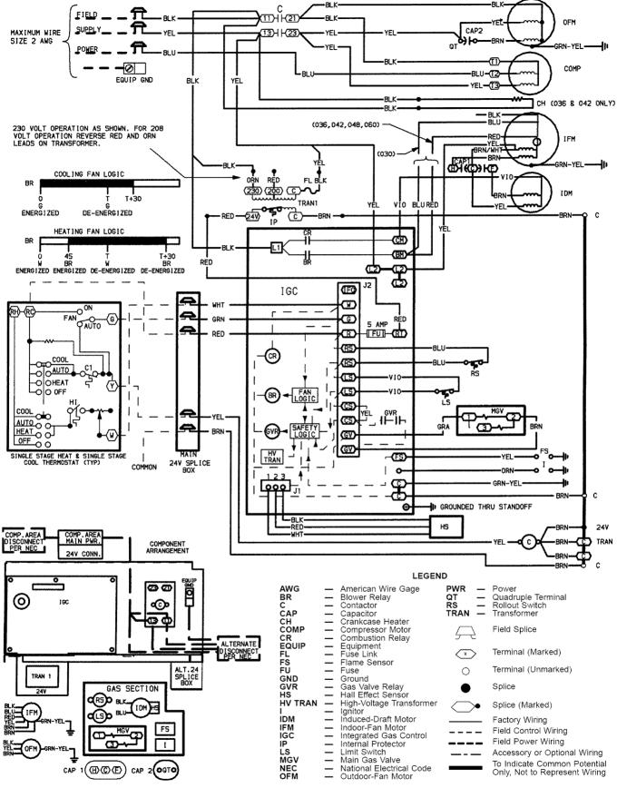
If any of the original wire furnished must be replaced, it must be replaced with type 90 C wire or its equivalent. 1
