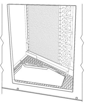
Fig. 14 — Vertical Duct Cover Removed
