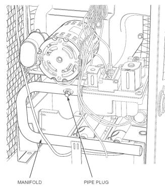
Fig. 19 — Burner Assembly
