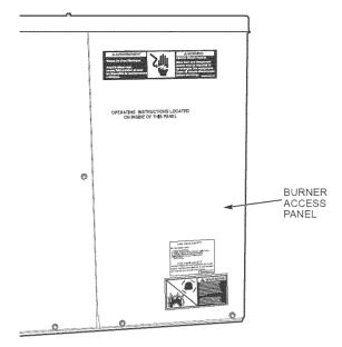
Fig. 25 — Burner Access Panel
