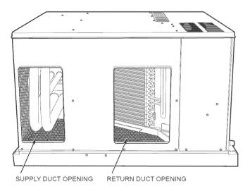
Fig. 12 — Supply and Return Duct Openings
