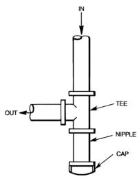
Fig. 11 — Sediment Trap
