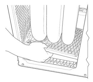
Fig. 15 — Removal of Vertical Discharge **Opening Cover**
