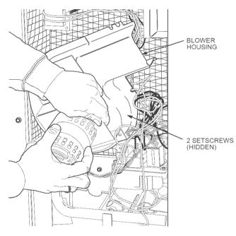
Fig. 26 — Removal of Motor and Blower Wheel
