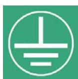
Cell Enhancers supplied from the mains must be connected to grounded outlets and earthed in conformity with appropriate local, national and international electricity supply and safety regulations.
