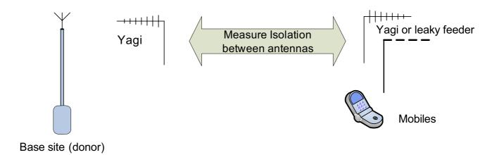
B). Install the Cell Enhancer with its gain set 10dB below the isolation figure obtained above.
