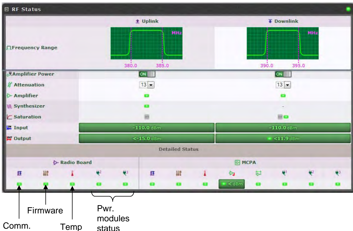
Figure 7-3: BSF-3604 Repeater Status
