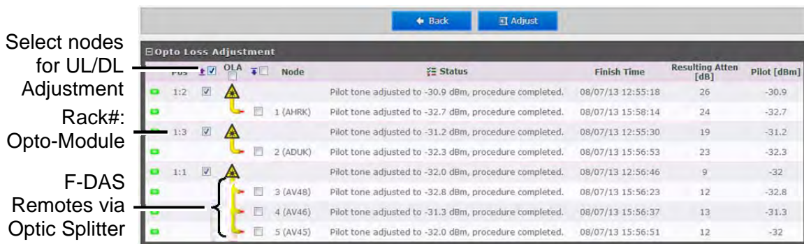
Figure 5-3. Configure and Initiate Optical Loss Adjustment
