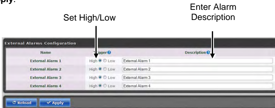
Figure 6-7: Configure External Alarms
