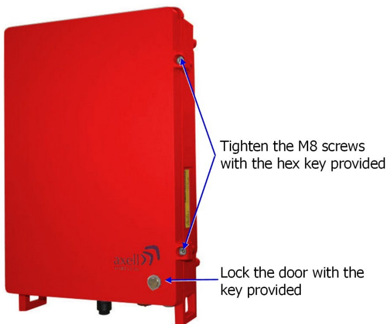
Figure 4-32: Securing the Repeater
