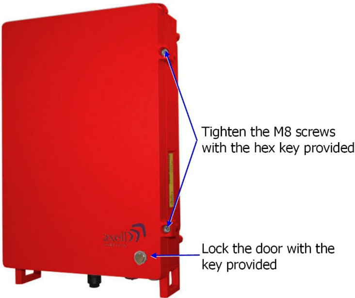
Figure 3-4: Securing the Repeater
