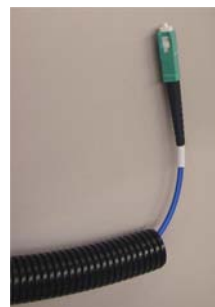
Figure 2-17: Run Optic Fibres through Sleeve
