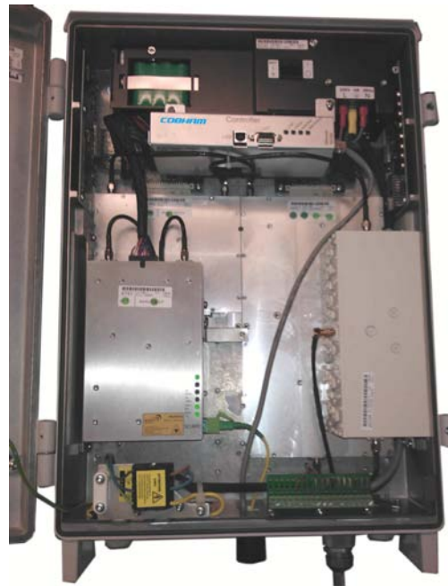
Figure 2-16: Example of Open Repeater Model
