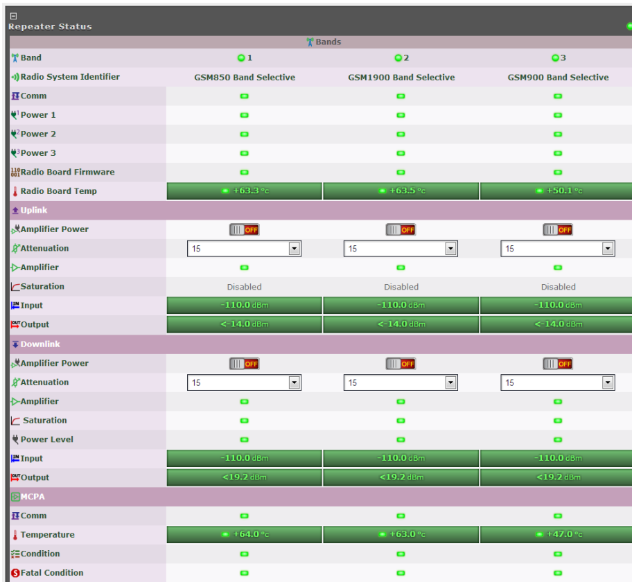
Figure 5-3: MBF-40 Repeater Status
