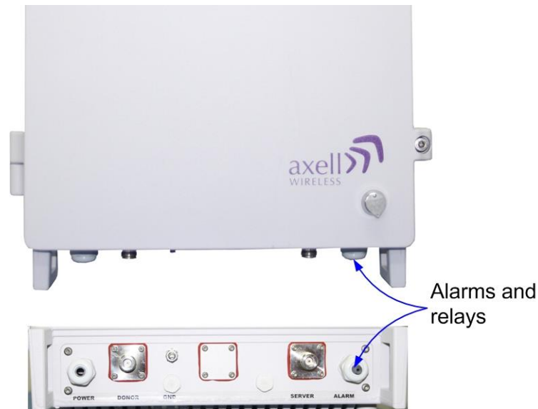
Figure 4-14. Alarm and Relay Connections
