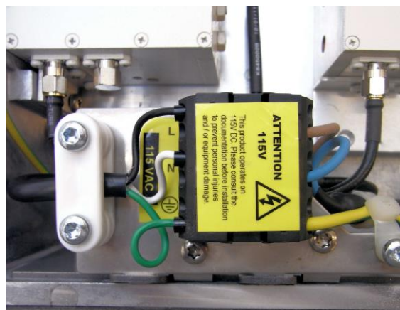
Figure 4-16 115V AC Power Source Connection
