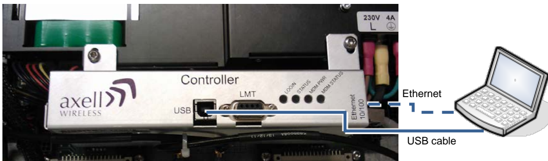
Figure 5-1: BSF-4004 Controller Module Connection
