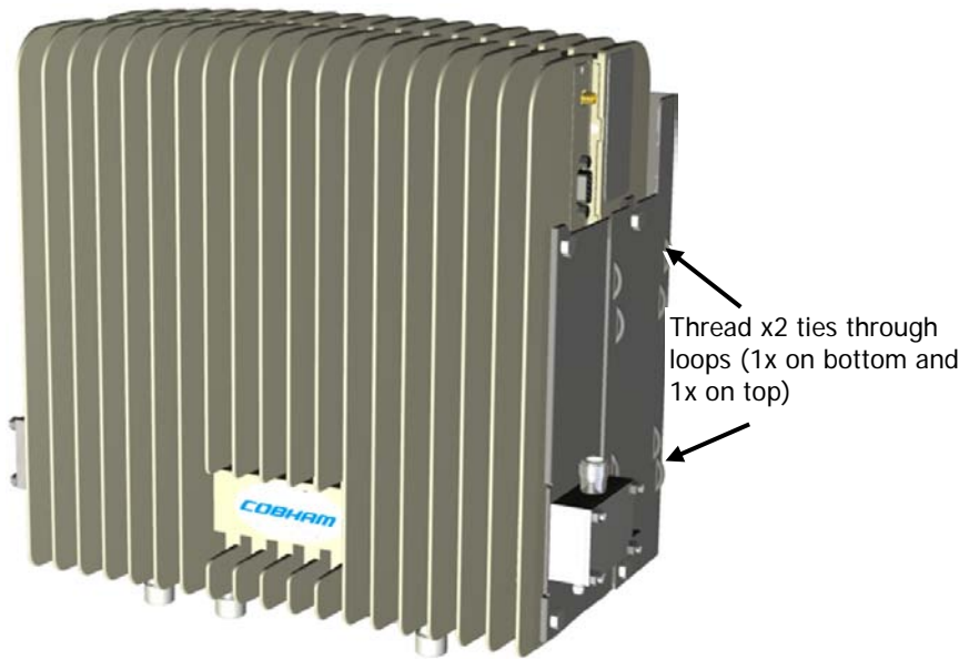
Figure 4-18. Insert Ties for Securing Power Supply
