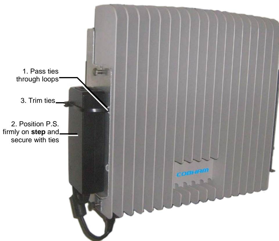
Figure 3-4. Mounting Power Supply
