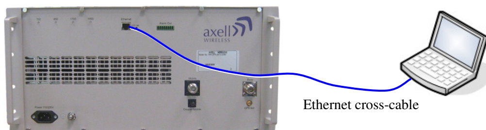
Figure 5.D-MBR-USA and Computer Ethernet Connection
