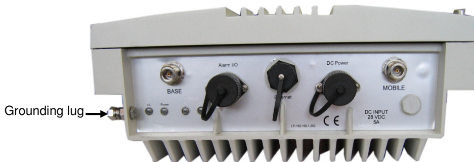
Figure 3-8. Grounding Lug Location
