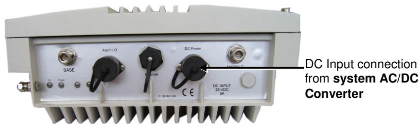
Figure 3-9. DC Power Input Connection Location
