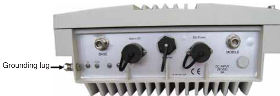
Figure 3-8. Grounding Lug Location
