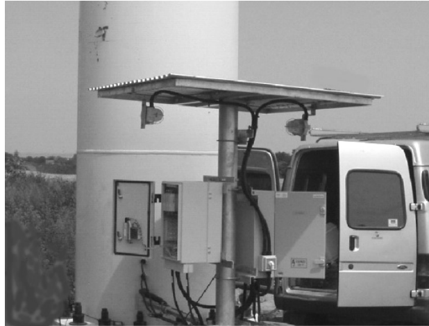
Figure 2-7: Example of a sun shield
