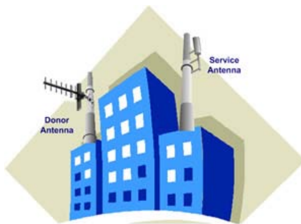
Figure 2-6. Service and Donor Antennas Installed on Opposite Sides of the Building
