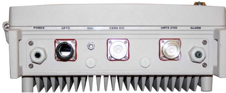
Figure 3-22: Grounding the MBF-40
