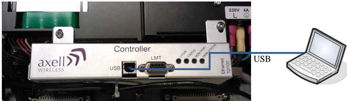
Figure 4-1: MBF-40 Controller Module Connection
