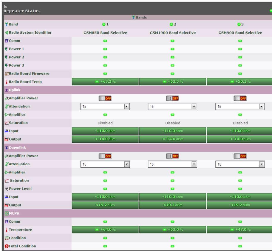
Figure 7-3: MBF-40 Repeater Status
