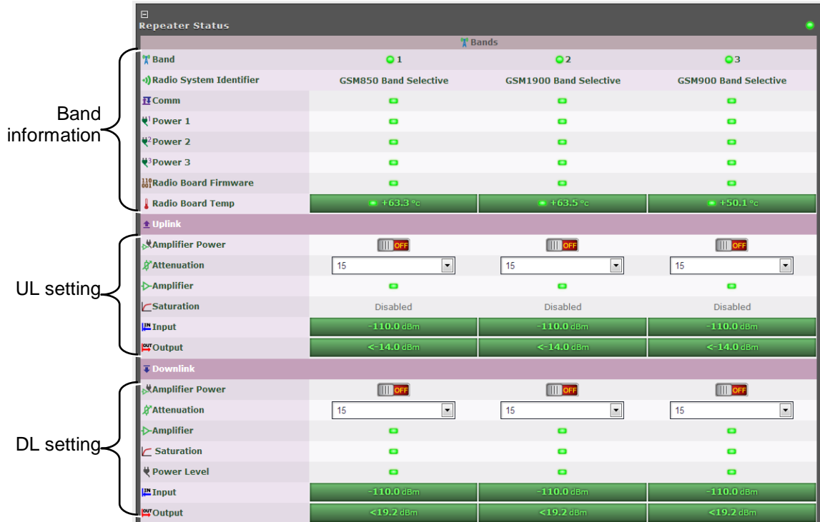
Figure 5-3: Example of MBF-40 Tri-Band Configuration window
