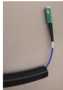
Figure 3-25: Run Optic Fibers through Sleeve
