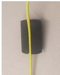
Figure 3-29: Run Fiber in the Rubber Seal (for MIMO, Run Both Fibers in the Same Rubber Seal)
