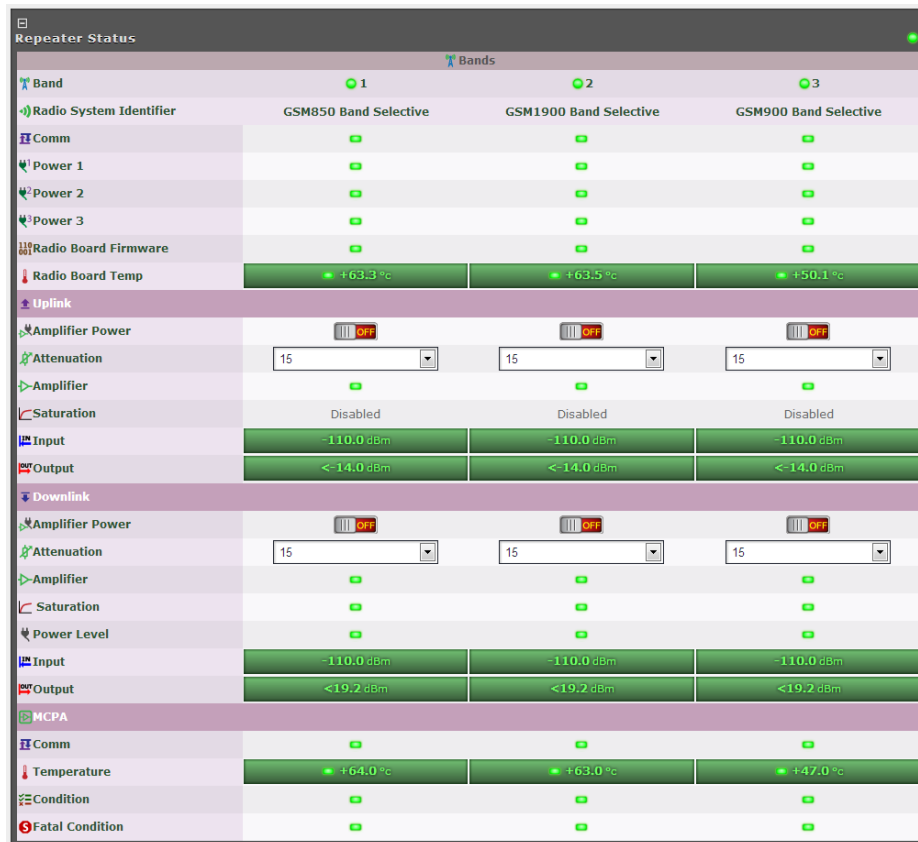
Figure 6-3: MBF-40 Repeater Status
