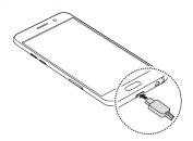
The charger should remain close to the electric socket and easily accessible while charging.
