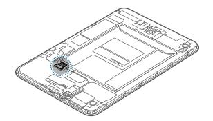
5 Peel the flap from the battery, and then pull it to remove the battery.
