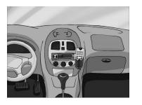
When installing the fixed mobile car phone avoid positioning the head control unit where it may disrupt the proper operation of the vehicle and/or its components, such as car stereo, air bags, cubbyhole, glove compartment, ashtray, lighter, gear stick, hand brake, etc ...
