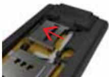
3. Lift the microSD card holder up with a fingernail and place the microSD card in the holder. Be sure the metal contacts on the card face the metal contacts inside the device. Also, be sure the shape of the card matches the holder exactly.
