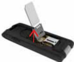
4. Push the inserted SIM card in the SIM card holder down and then slide it forward until the SIM card holder catches. Be sure the card is locked in place.
