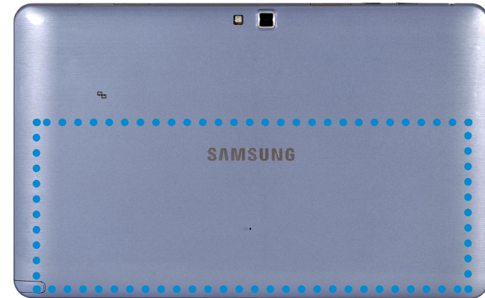
The location of the internal battery
