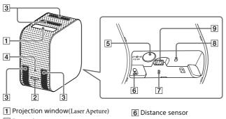
2 Power button 3 Ventilation holes (intake/exhaust)
