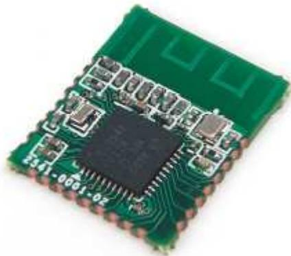
BT0001 build-in 8051 MCU, in-system software stack programmable flash memory, 8-KB RAM, and many multiple configuration options other powerful supporting features and peripherals, including UART, IIC and GPIO.
