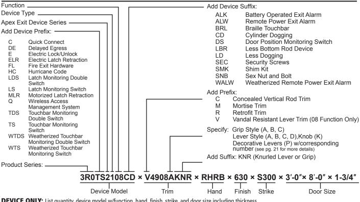
**DEVICE ONLY:** List quantity, device model w/function, hand, finish, strike, and door size including thickness. Note: For greater exit device mounting heights, see extended bottom rods (pages 35, 36, 37 & 38)
