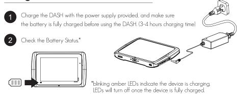
To turn on the DASH, press and hold the Power button for 3 seconds (Not the Home button)
