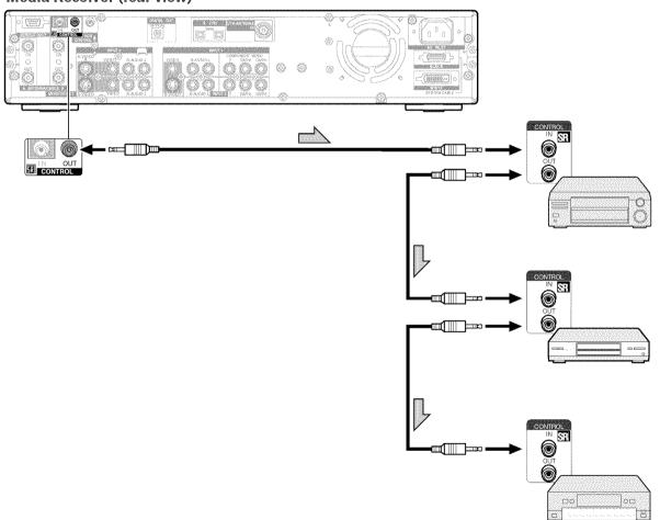
The control cables (commercially available) are mono sound cables with mini plugs (no resistance).
