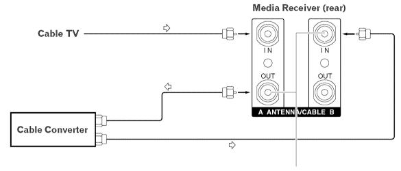
When making the above connections, first remove the coaxial cable attached before shipment.
