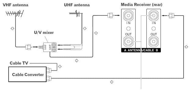
When making the above connections, first remove the coaxial cable attached before shipment.
