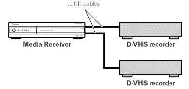
Using i.LINK cables you can also connect up to two D-VHS recorders in a daisy chain.
