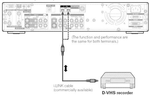
To use i.LINK, you need to connect only an i.LINK cable; you need not connect cables to the video and audio terminals.
