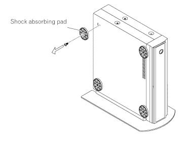
Keep the shock absorbing pads and screws. They are required when you place the Media Receiver in the horizontal position.
