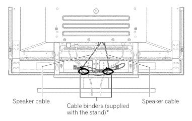
\* Cable binder Using the cable binders supplied with the stand, put the speaker and system cables together so that the cables are invisible from the front. At that time be careful not to apply any force to the connection sections of the cables.
