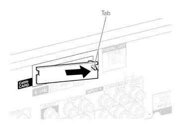
**3** Insert the specified cable card into the Cable CARD slot as far as it goes.
