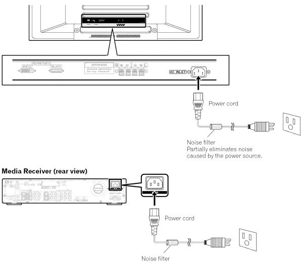
Partially eliminates noise caused by the power source.
