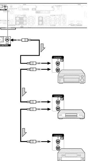
The control cables (commercially available) are mono sound cables with mini plugs (no resistance).
