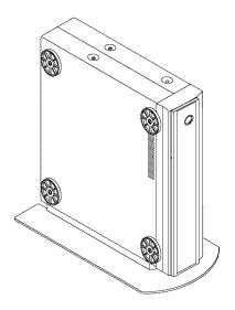
3. Remove the shock absorbing pads.
