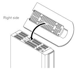
2. Secure the stand with the supplied screws.
