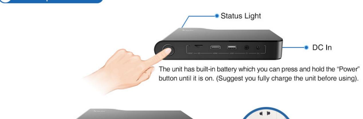
Or you can charge the battery and use the projector by plugging in the socket with our supplied adapter.
