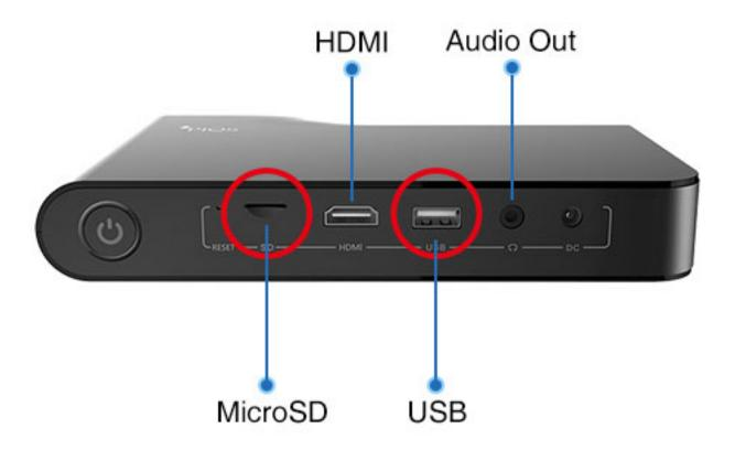
The unit has external slots for USB and MicroSD which you can playback photos, videos or documents directly. Open those files depending on the Apps installed.
