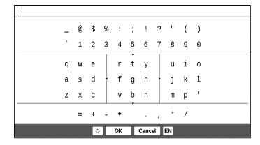
To work with the keyboard buttons "Up", "Down", "Left", "Right" and click "OK". To speed up the work with the keyboard all the characters are divided into 5 zones. The first button executes a rapid transition in the middle of the selected area, then you can select the desired character of this zone. To switch the
