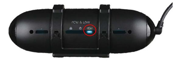
• **READY LED :** This LED will be turned on when the GPS is normal and sends the speed signal to Roadscope LX. The LED light is blue color.
