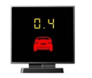
In the case of the third warning with the vehicle speed above the FCW threshold setting (Red vehicle icon with TTC) The third TTC start point is fixed.
