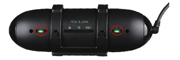
LDW LED : LDW LED will be turned on when the driver's vehicle is driven over the speed which is set(Default LDW speed value is 60km/h). In case of lane departure, it will blink. If the driver uses turn signal, the LED will be turned off. The LED light is green color.
