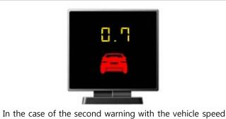
In the case of the second warning with the vehicle speed above the FCW threshold setting (Red blinking vehicle icon with TTC) The second TTC start point can be changed through the manager program or smart phone App.
