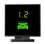
In the case of detecting the preceding vehicle with the vehicle speed above the FCW threshold setting (Bright green vehicle icon and TTC)
