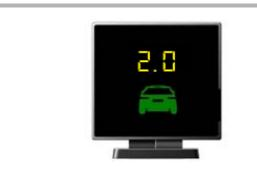
In the case of detecting the preceding vehicle with the vehicle speed above the FCW threshold setting (Dark green vehicle icon when exceeding TTC 2.0)
