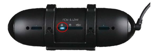
FCW LED : This LED will be turned on when the driver's vehicle is driven over the speed which is set (Default FCW speed value is 20km/h) and the device will detect the front vehicles. In case of collision risks, it will blink. The LED light is blue color.
