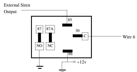
**Note**: The connection numbers correspond to the BOSCH 12V 40A relay.
