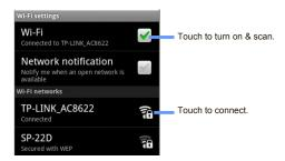
Turn Wireless Connection on or off Find it: Menu 🔀 > Settings > Wireless & networks > Wireless Connection. Note: To extend battery life, turn off Wireless Connection power when not in use.
