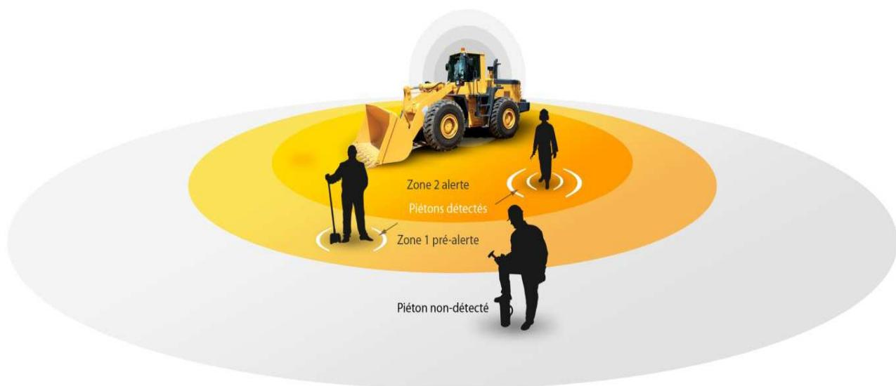
The SaveXSA-IHM device's display installed in the driver cab indicates the number of pedestrians detected in the pre-alert or alert zones.
