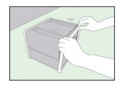
• Insert tray using the guide rails on either side of the unit as shown in the visual opposite.
