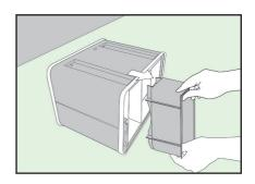
Using the screwdriver provided, fix the fascia panel onto the tray using the screws as shown in the visual opposite.
