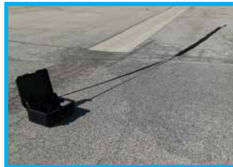
Figure 11. Extended Sleeve and Drogue
