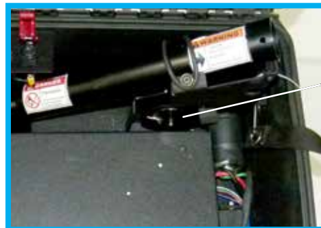
Figure 26. Exposed Spool Screw
