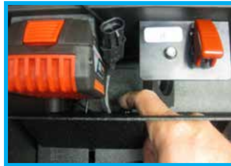
Figure 24. Locate Reset Button Facing the Power Switch
