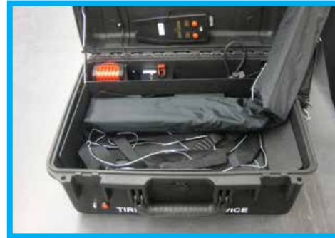
Figure 16. First Spike strip With Tether to the Left Side
