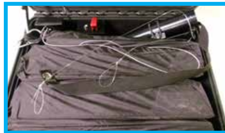
Figure 23A. Launch Tube Lines Before Attachment to Drogue
