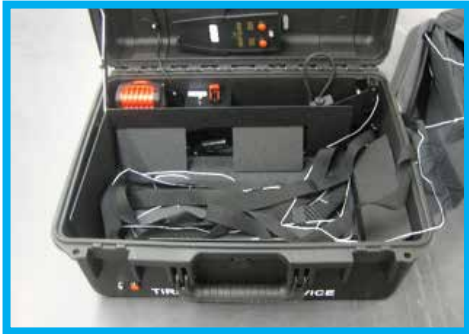
Figure 15. Tether and Retraction String Layered in Tray
