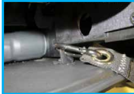
Figure 12. Attach Tether to Retract Bracket
