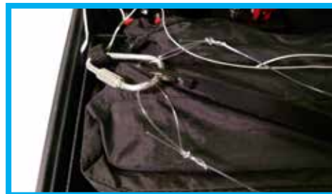
Figure 23B. Launch Tube Attachment to Drogue Clip
